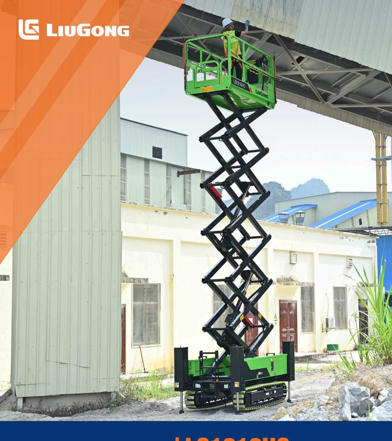
Working Height Max. Lift Capacity Max. Overall Width Overall Length Overall Weight 14 m (45'11") 320 kg (705 lb) 1.56 m (5'1") 2.8 m (9'2") 3,700 kg (8,157 lb)
